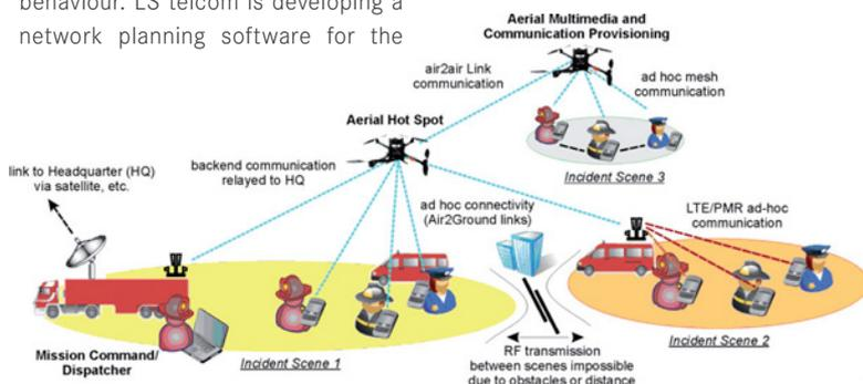
Picture: Ad hoc communication using UAV supported mesh and ad hoc cellular networks
