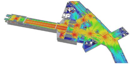
Coverage simulation for underground station with tunnel system
