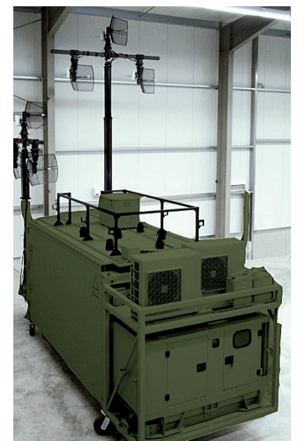
Sheltered EW operations center
